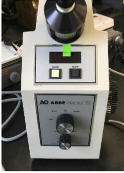
**Figure 6:** Refractometer (ABBE Mark III)
